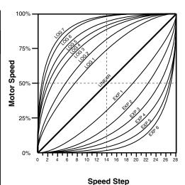
The exact throttle response for each curve is shown graphically. The logarithmic curve provides a rapid throttle response at low speeds, while the exponential curve provides a rapid throttle response at higher speeds.
