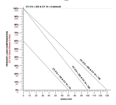
In general, you will want full load compensation at low speeds which gradually reduces to zero load compensation at full throttle and may be achieved by setting CV 10 to 126.
